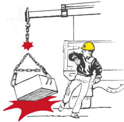
Figure 8.6: Use gentle lever movements to avoid shock loading.
