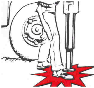
Figure 7.10: Keep limbs away when deploying or retracting stabilizers
