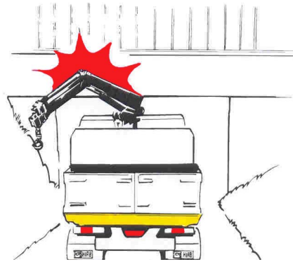
Figure 8.14: Always travel with the crane properly stowed.
