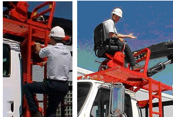
Figures 3.5a & 3.5b: Top Seat Control Station
