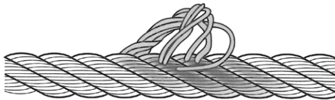
Figure 13.7: Example of protruding wire core
