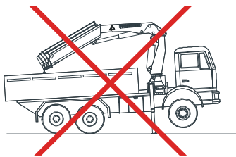
Figure 7.12: Keep all steering and drive tires on ground when setting up stabilizers
