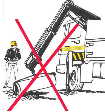
Figure 8.11: Never drag a load sideways
